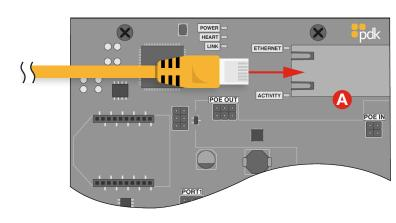
A Ethernet - Red controllers accept RJ45 connections. The Red 2 controller will be Self-Discoverable from Pdk io software. You have the option to assign a Static IP address but is not required.
