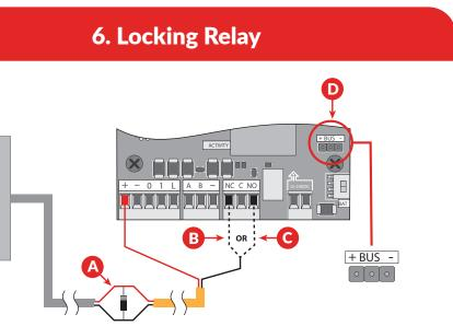
**Diode** - The provided diode must be installed when using a strike. Install at the strike with the grey stripe of diode on positive and the black on nega-
