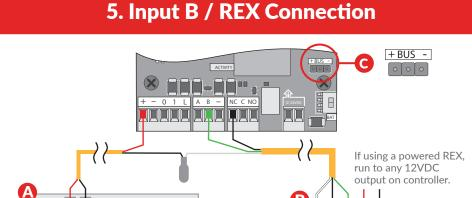
**Maglock** - When installing a Maglock it is typical to install a REX (Request to Exit) at the door for free egress. Run an 18/2 wire from the Maglock to the Door Controller, connecting to the Maglock as shown.
