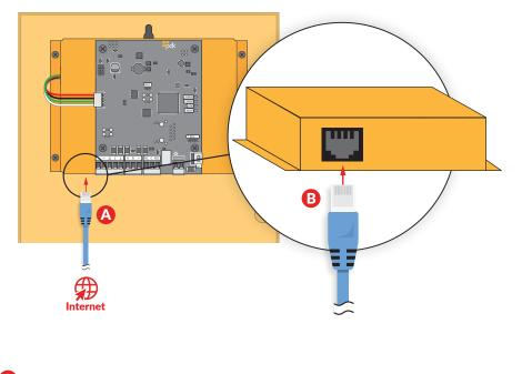
A Network - A live Internet connection is required to program and manage the Red Cloud Node.
