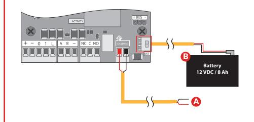
A DC INPUT - Use included 14 VDC, 2 amp transformer for DC power input. It is recommended to use 18/2 wire. For high voltage applications, use the HV Converter (PN: HVC).
