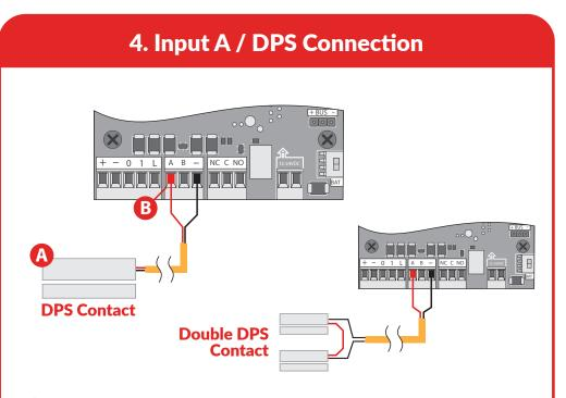
**A** DPS (Door Position Switch) - The DPS is mounted on the door frame in the desired location with a 22/2 wire running from the DPS to the controller. Wire the DPS to the controller as shown above. When using two DPS sensors for double doors you will wire them in series with only two conductors running back to the controller for connection.
