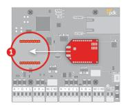
1 Plug the wireless module into the Red 2 board as shown in the image.
