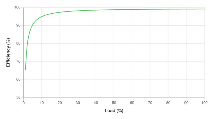
Curve fit of data measured in accordance with the US DOE Test Procedure for Uninterruptible Power Supplies. All measurements taken in normal mode(s), at typical environmental conditions, with 120V/60Hz electrical input and balanced resistive load (PF = 1.0) output.
