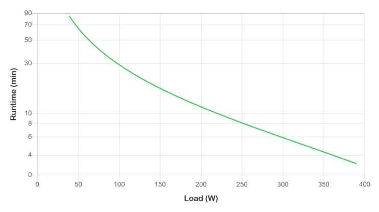
This graph is based on actual measured runtime data. All measurements were taken with new, fully charged batteries and a balanced resistive load (PF = 1.0). Actual runtimes may vary from the values of this graph. Actual runtimes are dependent on several v
