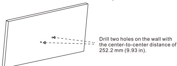
Note: If the router is installed on a wall, the expansion anchors and screws are customer-supplied.
