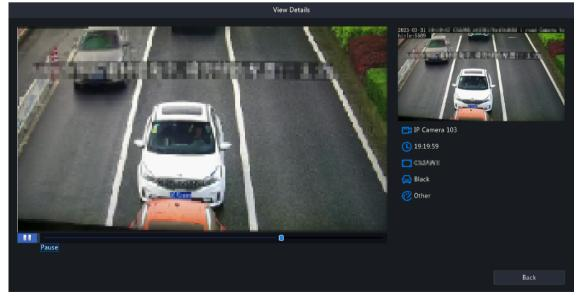
In the **View Details** dialog box, a 15s video (10s before and 5s after the snapshot time) is automatically played on the left, and the snapshot and its detailed information including camera name, time, license plate number, vehicle color, and plate color are displayed on the right.
