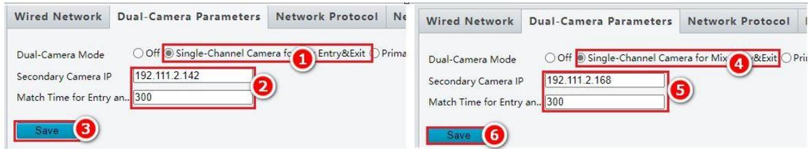
1. Log in to IPC1's web interface, choose **Setup > Network > Dual-Camera Parameters**. Select **Single-Channel Camera for Mix Entry&Exit**.
