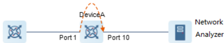
Figure 3-5 Operating Principle of Port Mirroring
